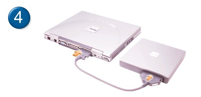
Connect the media bay cable to the external media bay and to the external media bay connector on the back of the computer.
